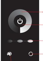
When you touch the color wheel, you will switch to the static brightness on the touch ring, regardless of whether you are in static or dynamic mode. In any state, the controller output can be turned on or off; When the controller is on, press and hold it button for more than 3 seconds to turn the output of the buzzer on or off.
